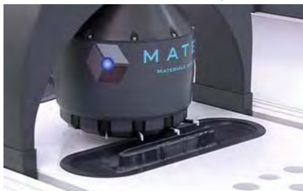
Figure 3. Image of MATECH's side-contact chuck (CAT chuck). Notice the position of the fingers that have moved out of the way to avoid contact with the etching fluid while the remaining fingers stay in contact with the sides of the thin wafer keeping it within capture range of the fluid pool. The adaptive handling allows the chuck to manage ultrathin, severely distorted wafers while making no contact with the non-process side.
