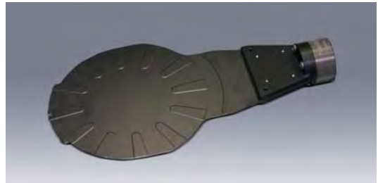
Figure 5. Bernoulli end effector effectively and consistently handles unsupported ultrathin wafers, down to 50µm thick. This image shows an 8" end effector used in conjunction with a WaveEtch system equipped with a side-contact CAT chuck. The etching system handles and processes freestanding 6" and 8" ultrathin wafers.
